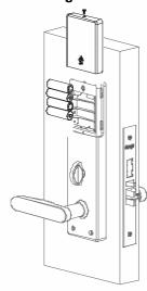
When the battery power is lower than 4.8v, there is beep sound for tip when you touch the card to open the door. you can still use around 100 times before the battery run out, so please change the battery in time!
