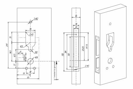
Find the below picture, please first draw one horizontal base line in the position of 1 meter to the ground, align the base line in the drill drawing with the drawn line and make the hole as the picture shows:
