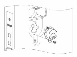
Remark: dot in the spindle shall align with the arrow in the mortise. Find below picture.
