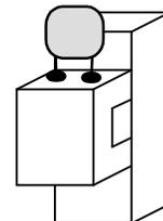
If you are using a « Shear Lock » electromagnetic lock, it is recommended to use a separate power supply than the one connected to the **PROMI/ECO** !
