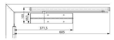
Space required on doors for standard installation on hinge side
