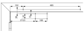
**Installation dimensions** for direct standard mounting on hinge side
