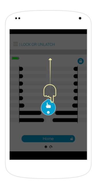
When the door is UNLOCKED SWIPE UP to lock it. Note: If the lock is set to Auto mode, the lock will lock itself automatically whenever the door is closed
