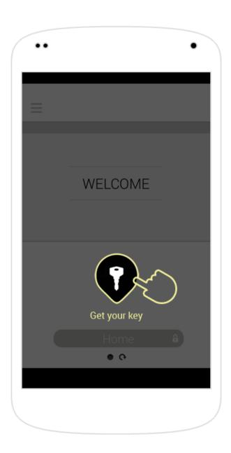
TAP the button to get your key. Note: Make sure your Bluetooth is on and that no other device is connected to the lock.
