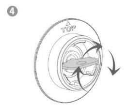
Use the Tightening Tool included to tighten the PeepHole barrel.
