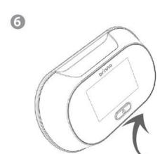
Rotate the PeepHole Viewer clockwise until horizontal and you feel it lock in place.
