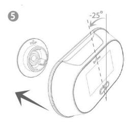
Hold the PeepHole Viewer at a -25 degree counter-clockwise position and insert it onto Base Flange.
