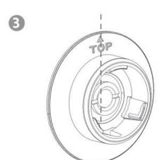
EN When the barrel is snug, rotate the Base Flange until the TOP icon is at 12 o'clock (vertical ).
