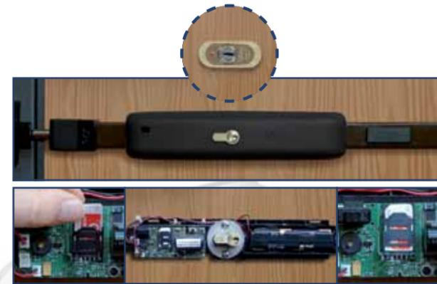
• By simply inserting a SIM card in the card holder in the special cover on the internal side, and by calling from your mobile phone (up to 5 different mobiles) the SIM card number, the numbers to be advised when an attempt is made to force entry will be memorized.
